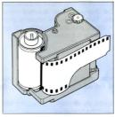
Set the film so that it surrounds the roller. pressure plate and sprocket.
